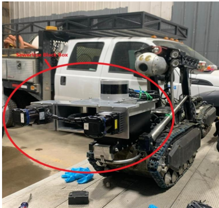
Figure 1: SewerVUE Technology Corp. "Black Box" on Pure Technologies Ltd. ROV.
